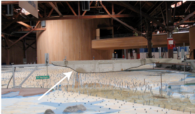
Figure 3: Model gate (indicated by arrow) used to simulate the dams proposed by Reber.
